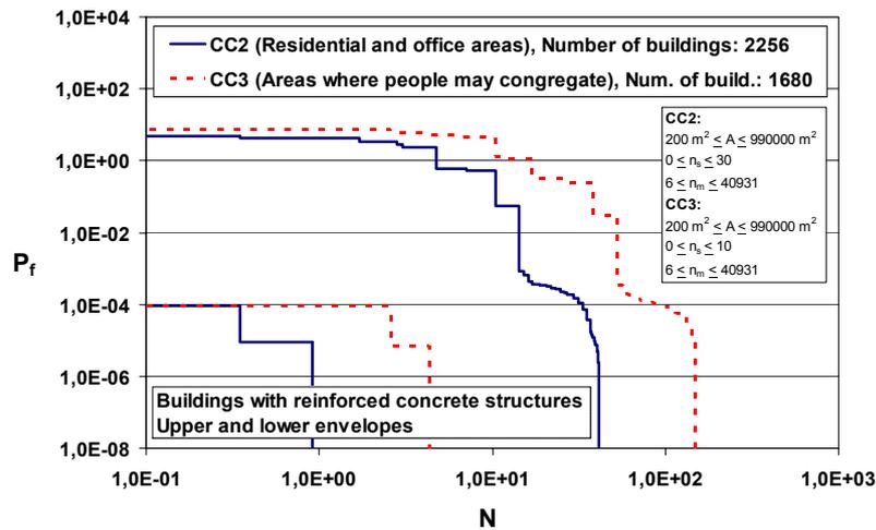
Figure 4: Upper and lower envelopes of the risk profiles for the buildings analysed with reinforced concrete structures ( $A$ : total net room area;  $n_s$ : number of storeys;  $n_m$ : number of structural members).
