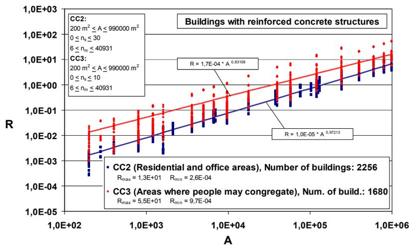
Figure 5: Collective risks to persons,  $R$ , versus total net room area,  $A$ , for the buildings analysed with reinforced concrete structures (Reference period: 50 years).
