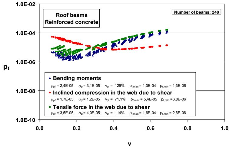
Figure 2: Probability of failure,  $p_f$ , vs. ratio of variable to total loads,  $v$ , for three failure mechanisms for each of the 240 roof beams analyzed (Reference period: 50 years) .
