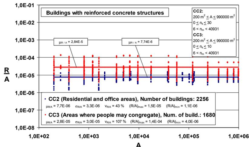
Figure 6: Collective risks to persons,  $R$ , standardized to the total net room area,  $A$ , versus  $A$ , for the buildings analysed with reinforced concrete structures (Reference period: 50 years).
